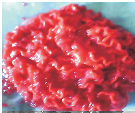
Fig. 3. Fungal mat showing adsorption of Rose Bengal Dye.
