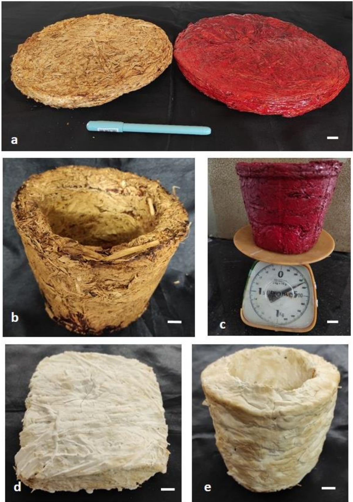
Figure 4: Products made out of biomaterial of spent mushroom substrate of P. ostreatus and P. tuber-regium fruit bodies grown in paddy straw. a, Product that can be used as packaging material; b, c, Flower pot made of SMS; d, Brick like structure; d, e, Products painted with cow dung paint. Scale bar = 1 cm.
