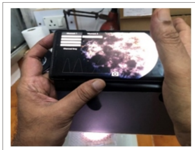
Fig.4: Direct Acquisition of images for stereomicroscopic characterization.
